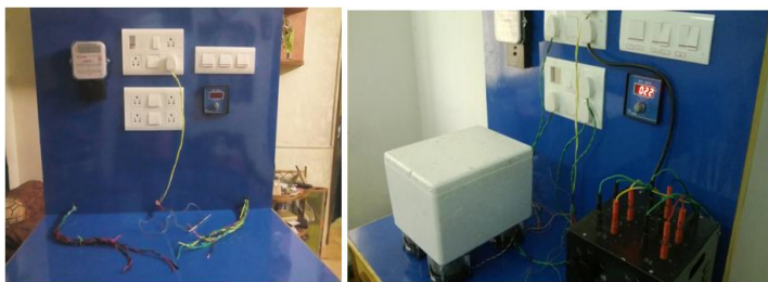
Experimental set-up with (a) Electrical circuit connections (b) transformer, modules, heat-sink and container connections
