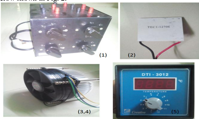
(1) Taping transformer (2) Thermo-electric module (3,4) Heat sink with fan (5) Temperature indicator
